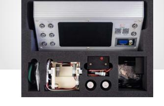
leXsolar H2 Expert offers a tabletop-sized experimental kit for the technical training of the Proton Exchange Membrane fuel cell systems. Due to the modular setup, the functionality of every component of the fuel cell system can be easily studied.
